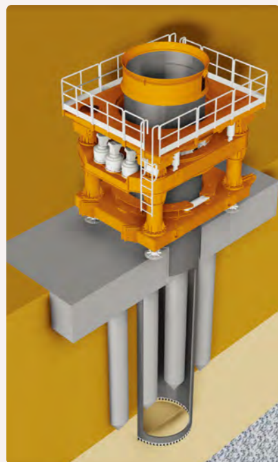
- Removing existing concrete piles
