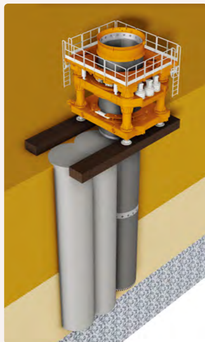
- Cutting through concrete in secant piling
