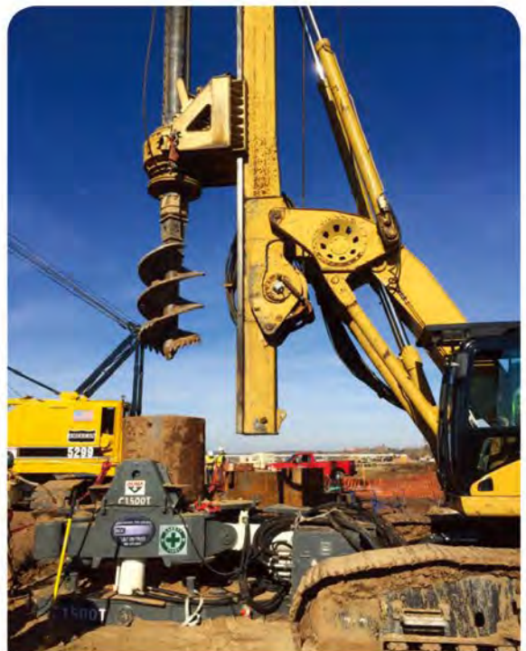
For drill mount oscillator (Tiny Model), It is required oscillator kit (Hooking lugs and Hyd. Ports to oscillator) to operate with the rotary drill rig.
