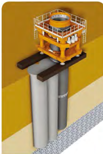
- Cutting through concrete in secant piling
