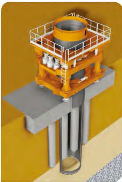
- Removing existing concrete piles
