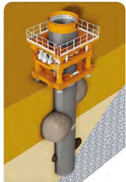
- Penetrating inclined rock layers or large boulders
